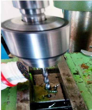
Figure 1: Drill done with the help of coolant
