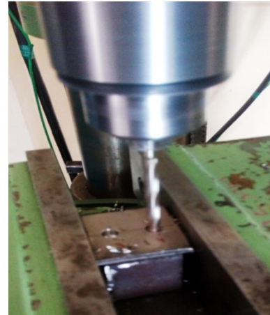
Figure 2: Drill done without the help of coolant
