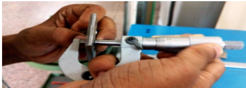
Figure 4: Measuring Burr Height through Micro Meter
